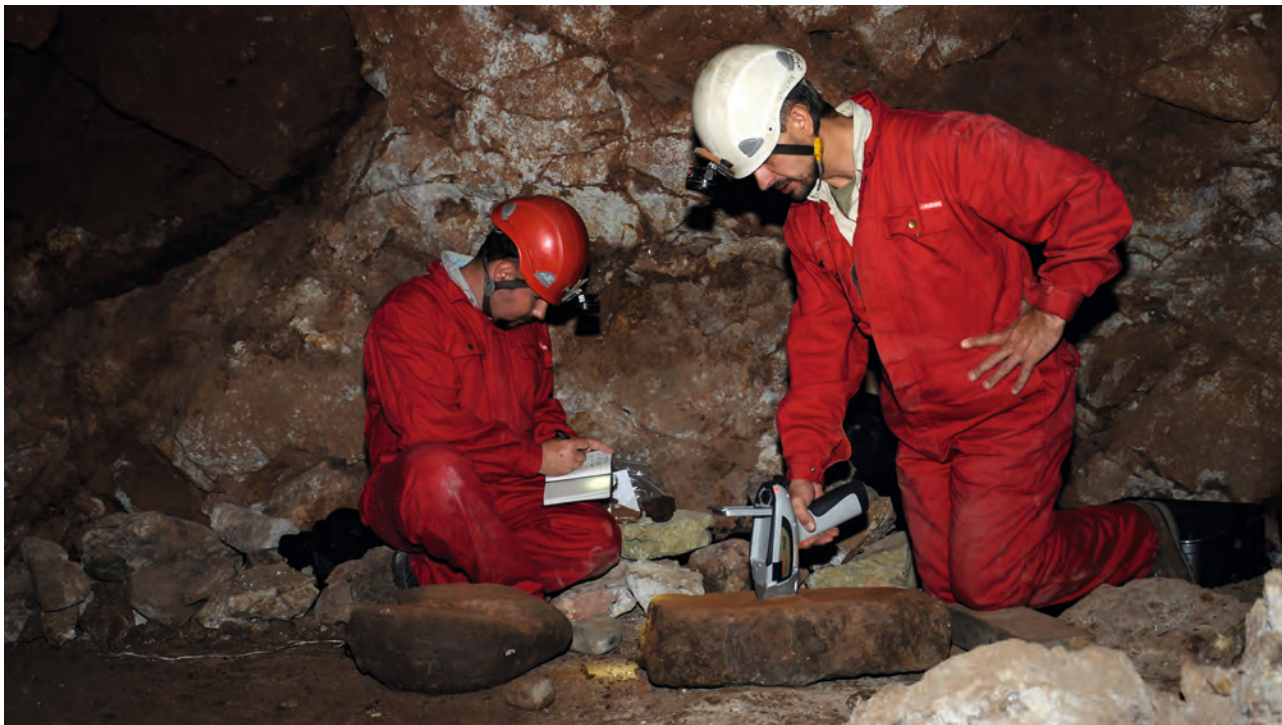
Testing the gold contents from ores in the gold mine of Sakdrisi; photo: F. Klein, DBM.
