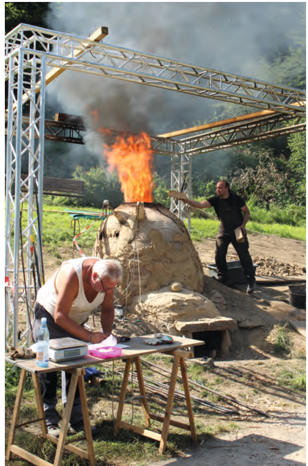
Smelting experiment, bloomery furnace; photo: M. Zeiler, LWL
