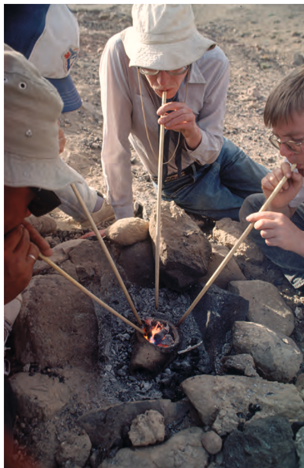
An experiment to reconstruct Early Bronze Age copper smelting in a crucible. Photo: A. Hauptmann, DBM
